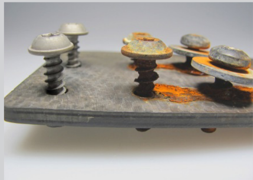
Comparison of b&m-CARBONPLAST® (left) with market-standard steel screws with Zn/Ni plating, (right) in the salt spray test after 480h
